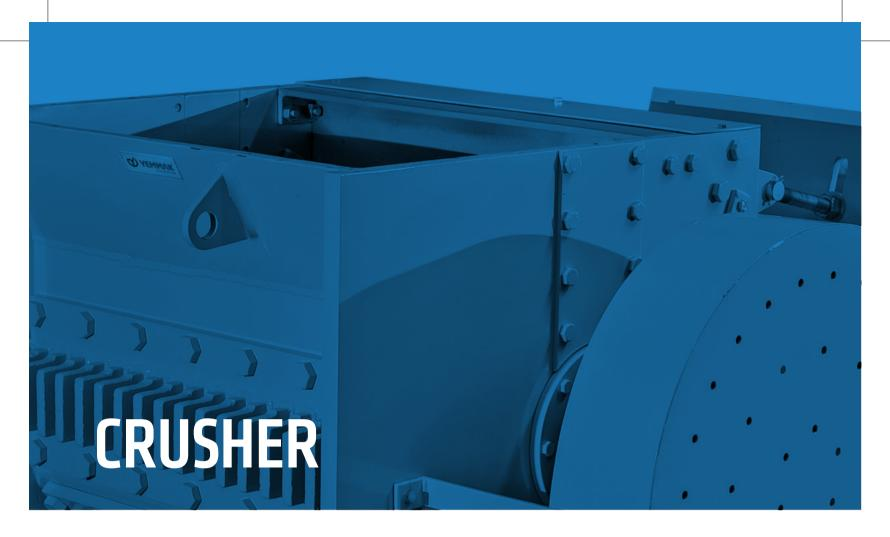
Yemmak Crushers are designed specifically for the rendering process and they can prepare animals' bones, offal, skeletons and the internal organs for the other stages of the process by effectively and homogenously shredding them.
